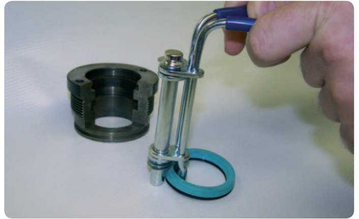
2. Proper tool positioning for grasping rod seal
